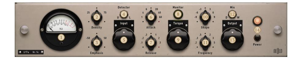
Shows either input level, gain reduction or output level (meter screw changes mode).
